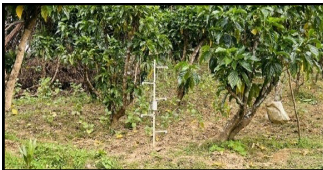
Fig. 35 IoT-enabled device for real-time microclimate monitoring and smart farming
